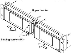
**4.** Fix the rear joint in place with binding screws (M3) to link the rear sides of the measuring instruments
