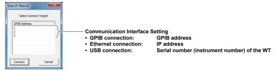
Select the communication interface setting of the power analyzer you want to use, and click Connect. A connection will be established with the analyzer.
