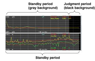
How the graph is displayed when the trend graph reaches the right edge of the display
