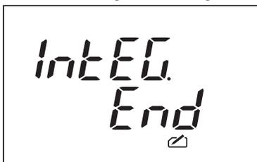
Pressing any key returns to the screen for instantaneous value measurement.
