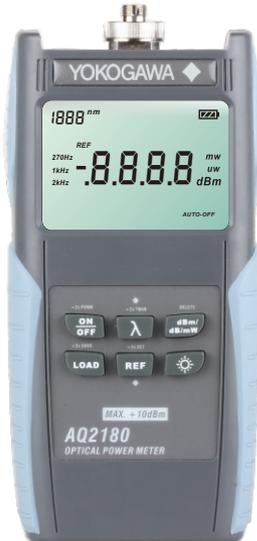
The AQ2180 series are full featured palm sized and lightweight optical power meters designed for use with an optical Light source to perform optical loss measurements on optical fiber cables.
