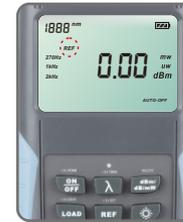
2. Press and hold the “REF” key over 2 seconds to store the presently measured value as the new reference value for the current wavelength. During the process the “REF” sign flashes twice on the screen and buzzer sound is heard. Once the new reference level is set, the AQ2180 switches to the dB measurement mode. The displayed value only lasts 1 second.
