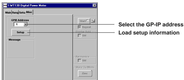
Select the GP-IB address of the WT130 with which you wish to communicate in the [GP-IB Address] list box. Click the [Setup] button to load the WT130's current setup information in the GP-IB window.
