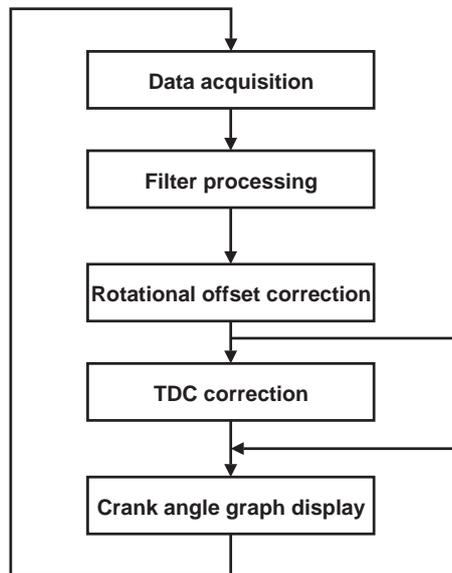
Rotational offset correction and TDC correction are the same process as in the Combustion Pressure Analysis Package.
