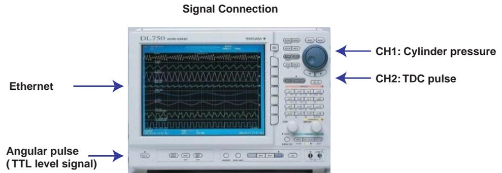
Connect an Ethernet cable to the main unit and turn on the power.
