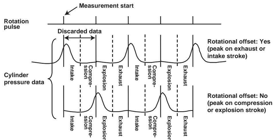
If the crank angle at the maximum point of pressure < -180 CA or if +180 CA < the crank angle at the maximum point of pressure, the rotational offset is set to "yes."
