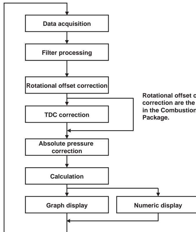
Rotational offset correction and TDC correction are the same process as in the Combustion Pressure Analysis Package.
