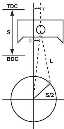
**9.  $V\theta$  [720]**Piston displacement ( $m^3$ )When **Clearance volume** is selected on the Parameter Settings screen
