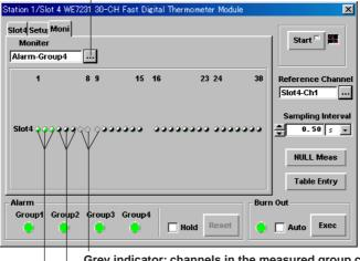
Grey indicator: channels in the measured group currently not being measured Black indicator: channels not set to output alarms
