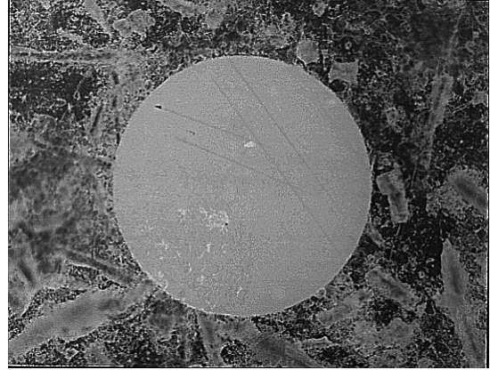
Enlarged photo of scratched optical connector connection part
