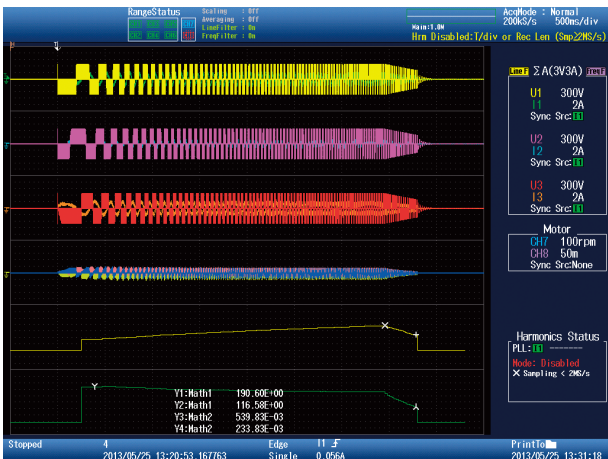
Figure 6. Example of the cycle-by-cycle trend calculation with the PX8000
