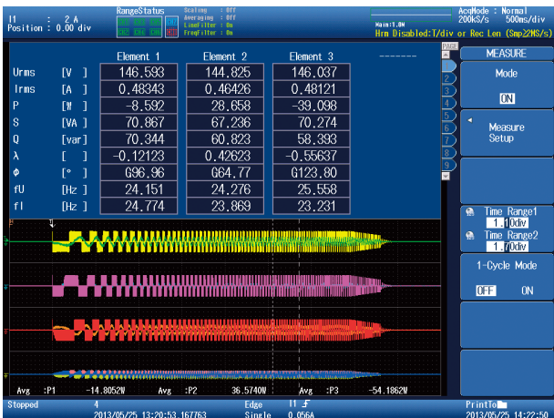
Figure 5. Example of the cursor interval calculation with the PX8000
