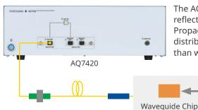
The AQ7420 series accurately captures sharp peaks, clearly resolving small reflections and scattered light near strong coupling-point reflections. Propagation loss can be calculated directly from the slope of the return loss distribution, enabling precise waveguide analysis at a lower cost and in less time than with the conventional cutback method.
