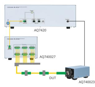
When paired with the AQ740027, the AQ7420/AQ7421 enables automatic inspection of multiple fibers and devices such as splitters. It can measure return loss and insertion loss simultaneously across multiple ports. This eliminates the need for manual reconnections or switching, allowing multiple ports to be tested with a single button press for maximum efficiency.
