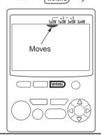
Moves to indicate the wiring method currently selected.
