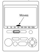
The current ranges that can be selected vary with the clamp-on current probe used, i.e., with the clamp setting.
