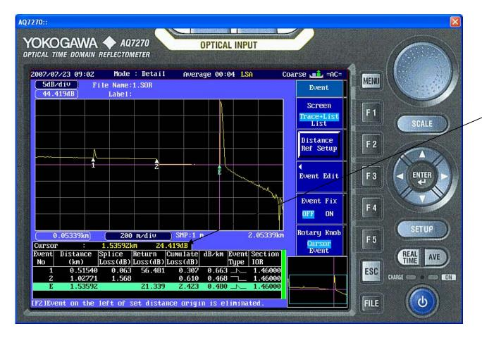
The Cursor value displays the level in dB that the signal is above the noise floor of the optical port you are connected to. The noise floor is basically the Dynamic range. This lets you know if you are approaching the maximum distance that you can test with the OTDR. As the cursor value approaches zero the OTDR is nearing its maximum measurable distance due to the condition of the fiber optic cable.
