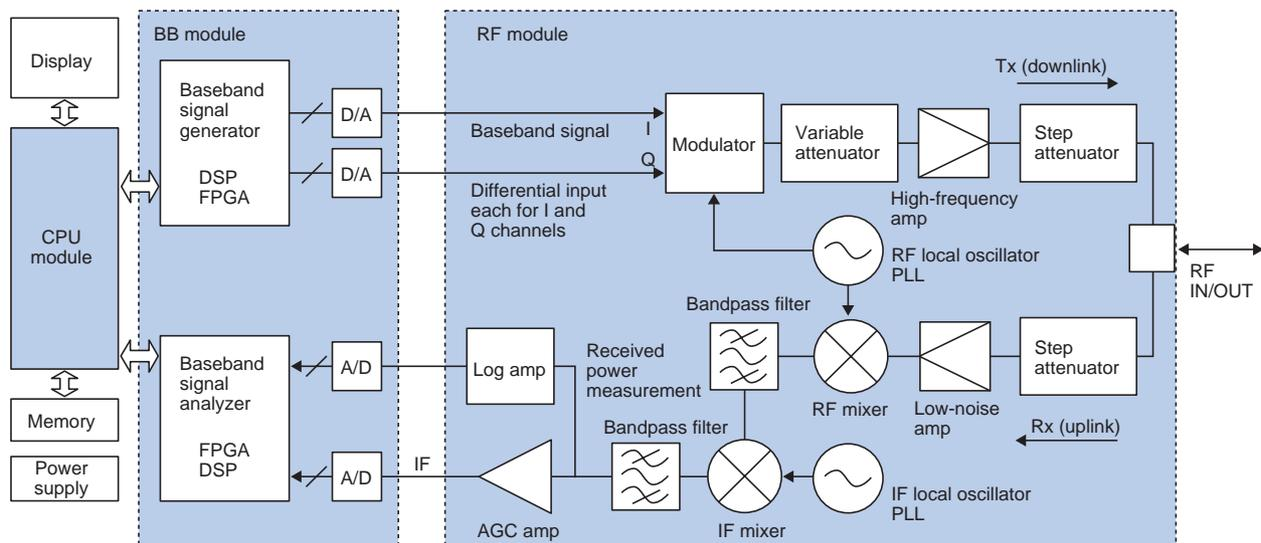
**Figure 2** VC200 Hardware Configuration
