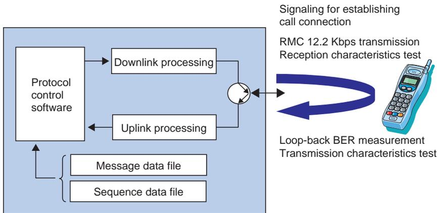
**Figure 3** W-CDMA Signaling Operations
