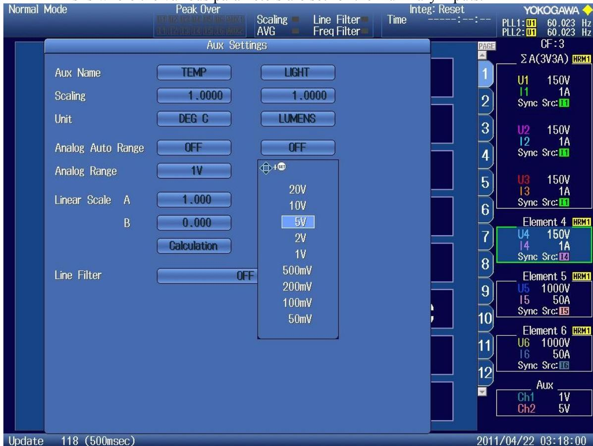
Use the Arrow Keys to move around the menu. Highlight the particular function, such as Range, and Press [SET] button to select. Use Arrow Key to highlight the desired Range and Press [SET] button to select.
