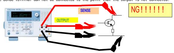
iv)Only GS820 has 2 channel. The CH2 of GS820 can measure the point that CH1 is not connected.
