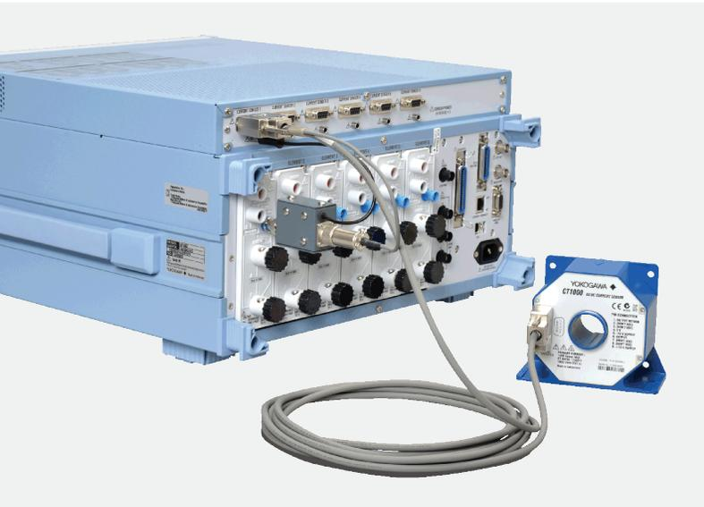
If you are measuring a current that does not exceed the maximum rated input current of the power analyzer you are working with, you can connect the current carrying cable directly to the current inputs of the power analyzer. Many times though, the current to measure will exceed the current input limits of your power analyzer. In these cases you can use a current transformer to convert the current to a voltage or current signal that can be measured directly by the power analyzer.
